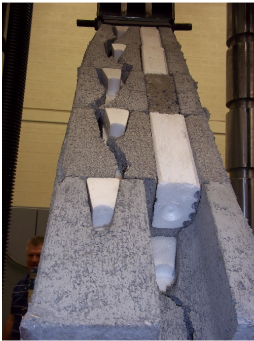
(a) Crack through webs.
