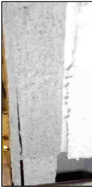
(a) Delamination of surface bond. (b) Typical cracks in face of wallette.
