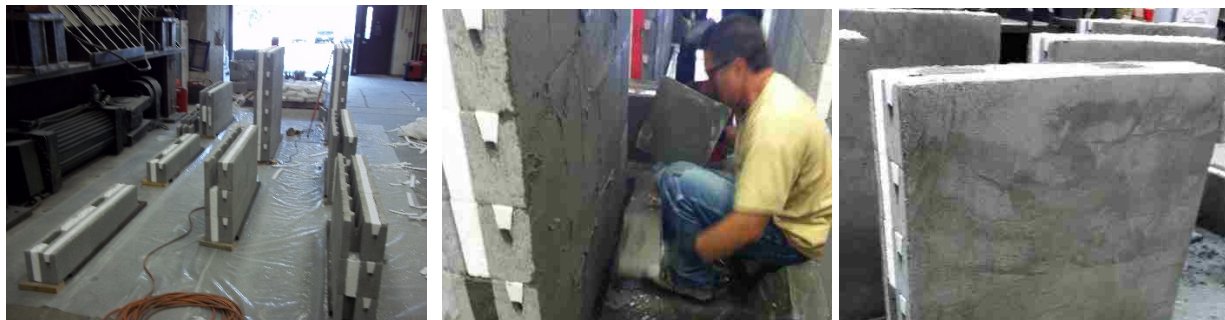
(a) Stacking the wallettes. (b) application of structural coat (c) Finished wallettes
