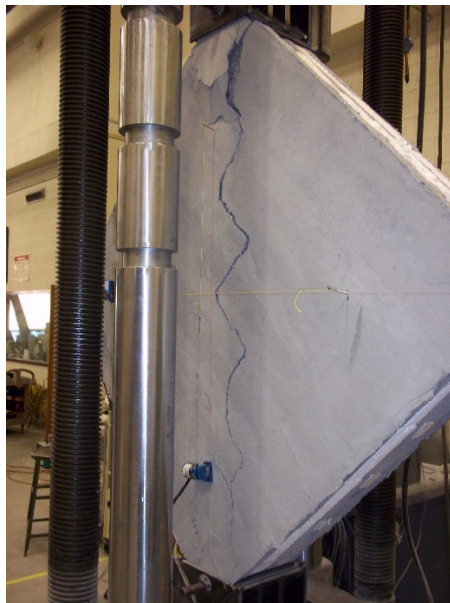
(a) Cracking of face of wallette.
