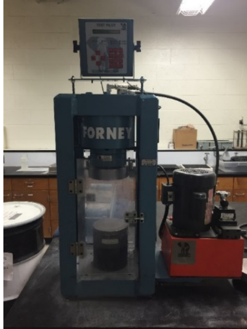
Figure 3-4 Forney Testing Machine.
