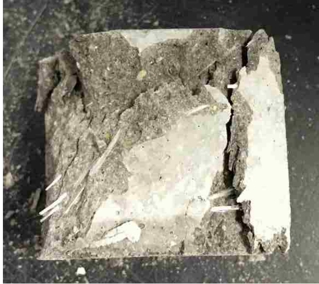
Figure 3-8 Typical failure of surface bond cubes.
