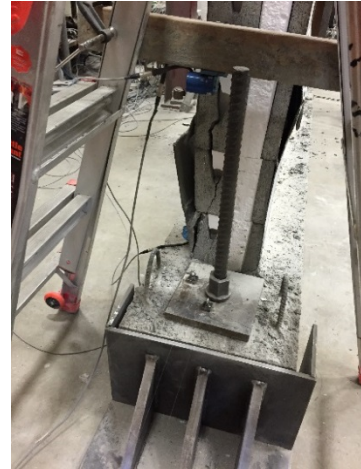
(c) Cracks in outer webs.
