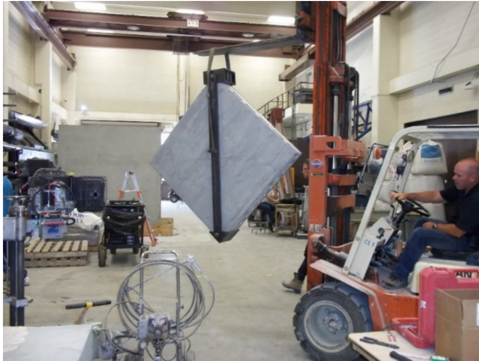
Figure 3-14 Transportation of walls during diagonal-tension test.
