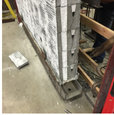
(b) Cracks in webs.
