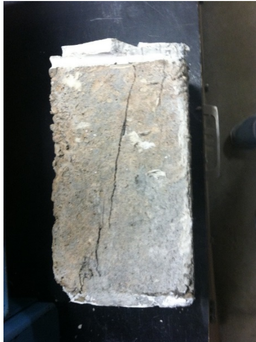
Figure 3-5 Typical failure of grout prisms.
