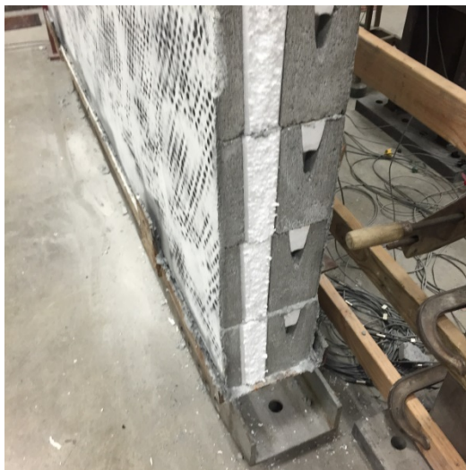
(a) No cracking in webs.
