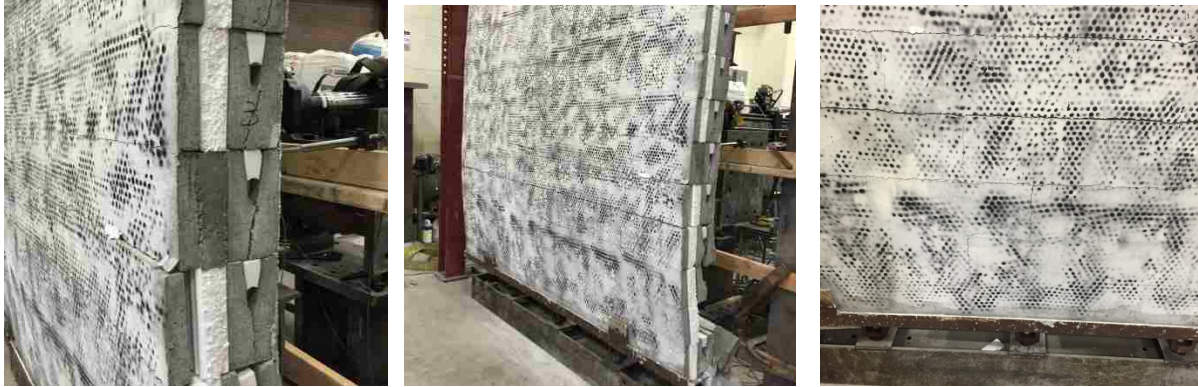
(a) Cracks in webs.
