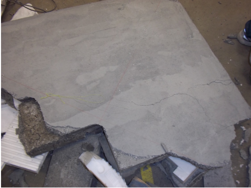
Figure 3-31 Wallette 8 after failure.
